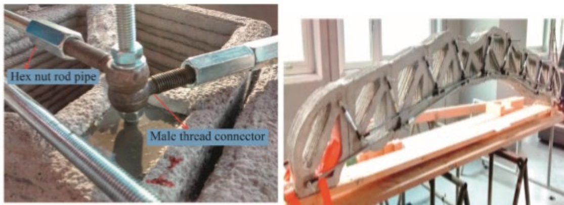
Figure 2.3 External Reinforcement Arrangement. (Asprone D., Auricchio F., Menna C., & Mercuri V, 2018). [15].
