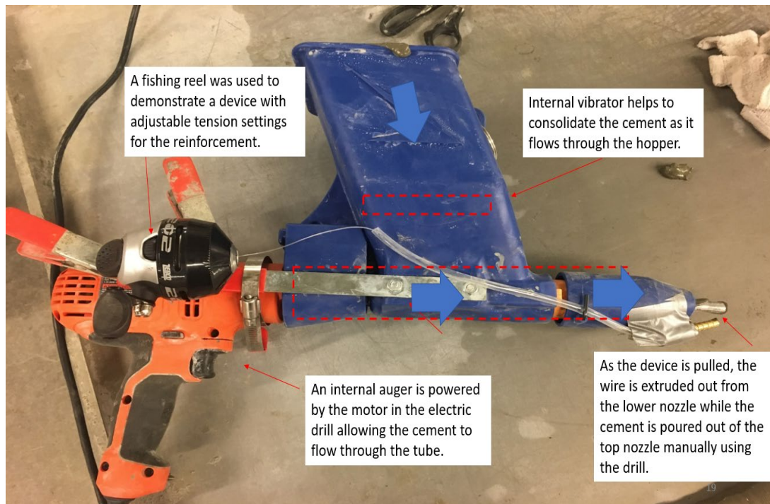
Figure 3.1 Mortar Gun (Manual Configuration).
